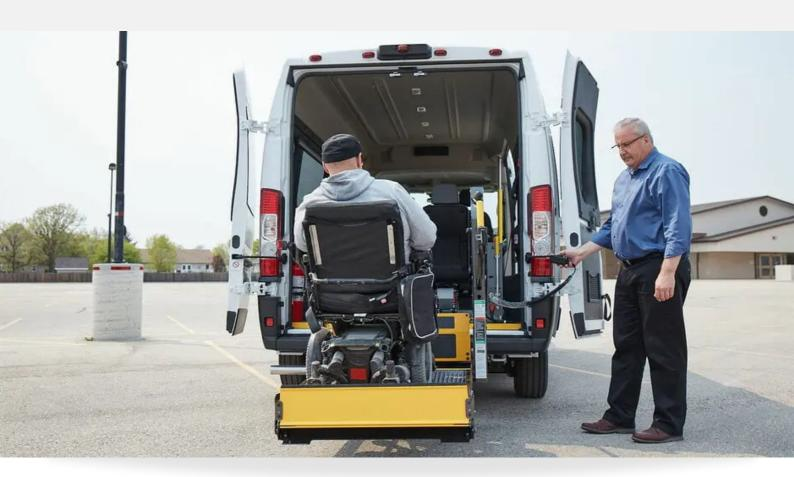
A wheelchair lift is a convenient and safe way for passengers to enter and exit a van.
