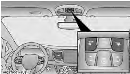
Courtesy Light Switches
