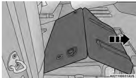
Extend Floor Panel
